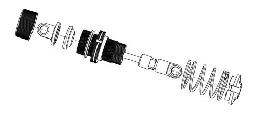
Close the shock absorber with rubber seal, ball joint and cap.
