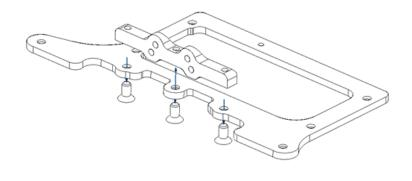
Using 3 x HW012 M3x6 countersunk screw to fix the Vlink2 to the motor pod
