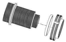
Lubricate and insert the o-ring into the setting ring.
