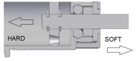
Take care when using conical pistons as shown.
