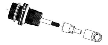
Screw together the M20-K7 droop adjuster and the ball joint (short)
