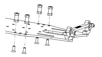
Assembly the 2 side dampers as shown. Use 30k syrup as starting point (not included)
