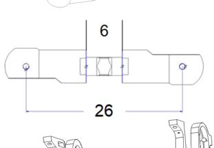
Build 2 sets of links using 2 x TR15 and 4 FX0037 - short
