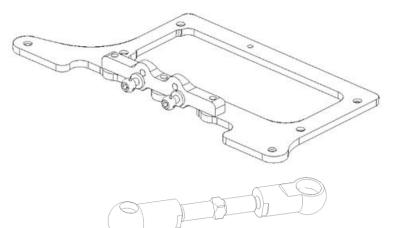
Insert 2 Fx0061-M ball studs in the V-link2
