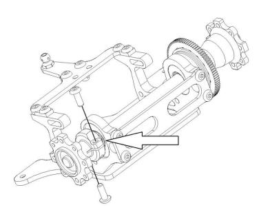
Slide the left hub HDD4 on the rear axle, leave 0.1-0.2mm of axial play. Clamp it on the axle using 2 x HW008 3x8 button screws
