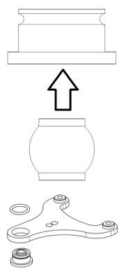
**Note:** Be sure that the sphere holder fit easily, you might have to enlarge the hole with some sandpaper.
