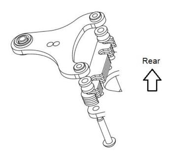
Insert the OPT-038 Oring around the sphere holder.
