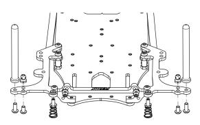
Assemble the FX-FU48 using 1 x HW008 3x6 button screw and the body post using 1 x HW007 3x8 button screw
