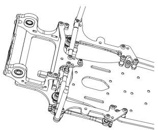
Insert the HW0029 M3x12 in the proper hole, then slide the G56-42-A spacer and the 1.5mm shim Install the link assembled previously
