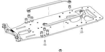
Locate the appropriate stiffener in the chassis bag.
