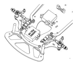
Following 1/12 servo can be fixed on the chassis: Power HD M8H or Sanwa PGS-HR or Power HD M8 (need G12 servo post – not included)
