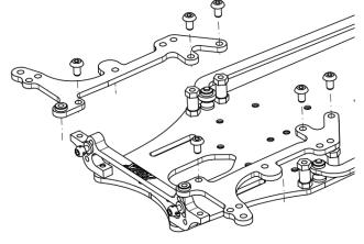
Using 6 x HW008 M3x6 button screws fix the 2 X G562-004 side wings on the 12mm posts and on the M20 V-Link1
