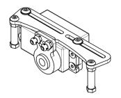
Fix the 2 x FX0052 20mm post to the servo holder using 2 x HW003 M3x8 button screw
