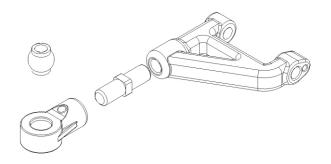
G56-031 arm – G56-033 eyelet-G56-032 turnbuckle G56-037 sphere
