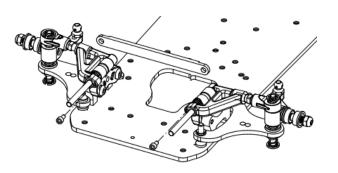
Slide the G56-013 front beam into the upper arm mounts, then insert the G56-034 hinge pins and secure them with the HW031 M2x4 screw
