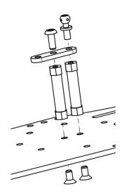
Fix 2 FX0054 26mm posts to the chassis using 2 M3x6 HW012 screws
