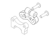
Secure the G56-030 upper arm mount to the G56-039 using 2 HW004 M3x10mm Hex button screw.
