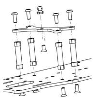
Fix 4 FX0054 26mm posts to the chassis using 4 M3x6 HW012 screws
