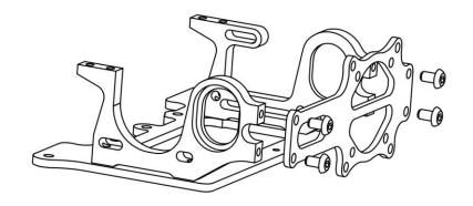
Fix the G562-201 brace to the group using 4 x HW008 M3x6 button screw. Tight the screws evenly using an "X" pattern
