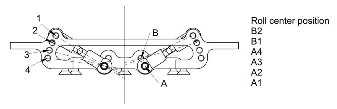
V-Link suspension has the unique ability to alter the roll centre position.
