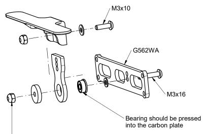
Adjust the tension using the M3 Nylock.
