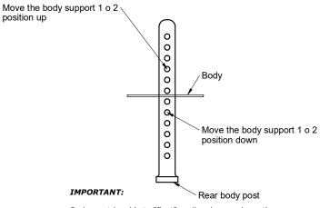
Body must be able to "float" easily, please enlarge the rear body holes 1-2mm
