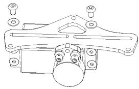
Fix the 3 x FX0052 20mm post to the servo holder using 3 x HW003 M3x8 button screw.
