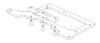
Using 3 x HW012 M3x6 countersunk screw fix the V-link2 to the motor pod.
