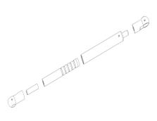
Assembly the 2 side dampers as shown
