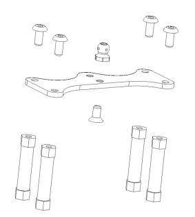
Fix the 4 by 26mm post using 4 x HW003 M3x8 button screw.
