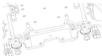
From Bag C, Insert 2 fx0024 ball stud in the V-link1 bridge.
