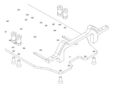
Take the 4 x FX0052 12mm post, the V-link 1 and 6 x HW007 M3x8 countersunk screw and assembly as shown.
