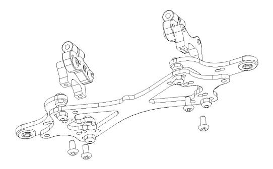
Assembly the 2 groups to the front bear with 4 x HW008 M3x8mm button screw. Use the innermost set of holes.
