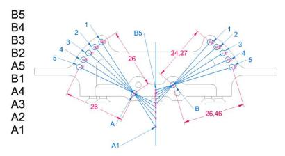
V-Link suspension has the unique ability to alter the roll centre position.
