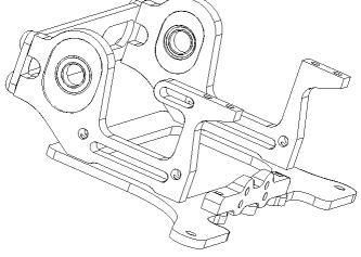
Insert the ride height adjuster and the flanged bearings (bearings might be located in the differential bag)
