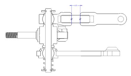
Set the distance at 4.5mm. Assembly the steering upright group as shown. Use the provided shims to fine tune the front ride height.
