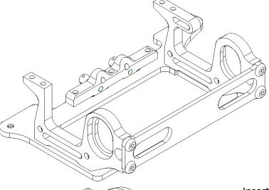
Fix the G56-021 brace to the group using 4 x HW008 M3x6 button screw.
