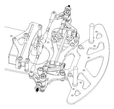
From bag B, use HW004 M3x10 countersunk screw and fix the Servo holder group.
