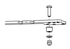
Insert the HW0029 M3x12 in the proper "A" hole, then slide the G56042-A spacer and the 1.5mm shim Install the link assembled previously
