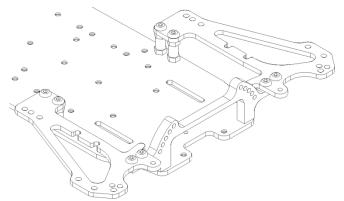
Using 4 x HW007 M3x8 button screws fix the 2 X G56-004 side wings on the 12mm posts. Use 4 x HW008 M3x6 on the V-Link bridge
