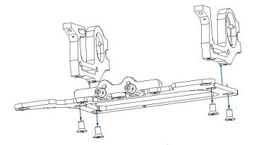
Using 4 x HW012 countersunk screws, fix the motor holder to the motor pod. Tight the screws evenly using an "X" pattern
