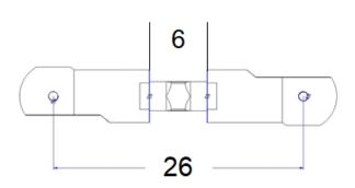
Keep this dimensions. Fix the link over the V-link2
