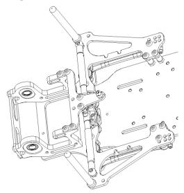
Using the parts remaining from Bag C Install now the 2 dampers and the shock holder using 4 x HW008 3x6 button screw.
