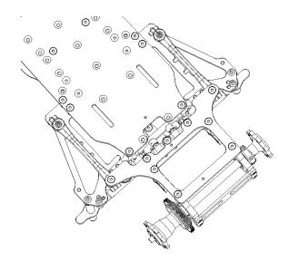
Fix the short link between V-link 1 and V-link2 Using 2 x HW006 M3x6 countersunk screw (from bag C), you can now install the link to the motor pod group.
