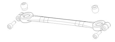
Use 2 x HW0014 M2x 6 screws and 2 x FX002 spheres each
