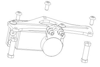
Be sure that the servo is centered. Keep the provided 3  $\times$  1.5mm shims and screws for a further step.
