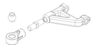
G56-031 arm – G56-033 eyelet-G56-032 turnbuckle G56-037 sphere
