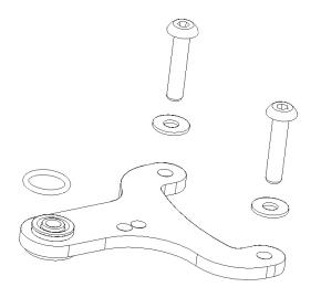
Insert the OPT-038 Oring around the sphere holder. Take 2 x HW018 M3 Washer and 2 x HW030 Me x 16mm button head screw. Make 2 sets mirror like
