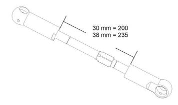
The dimension shown is a starting point, final refinement will be done while setting the model
