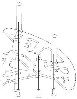
Fix the G56-006 bumper and fix it using 2 x HW004 M3x10 countersunk and 2 x HW002 M3 self-locking nut.
