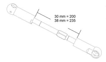
The dimension shown is a starting point, final refinement will be done while setting the model
