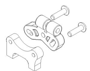
Secure the G56-030 upper arm mount to the G56-039 using 2 HW029 M3x12mm Hex button screw.
