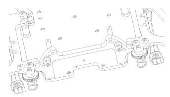
From Bag C, Insert 2 fx0024 ball stud in the V-link1 bridge.
