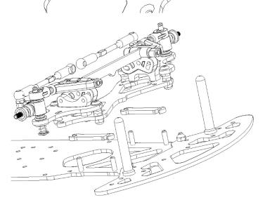
Take the 2 G56-016 2.5mm shims from Bag A, insert over the screws and slide the complete front end over the chassis. There are also 1mm and 0.5mm shims to set the front ride height.
