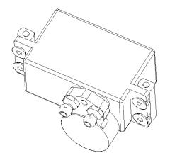
Assembled group. Servo saver should be vertical when servo is neutral.
