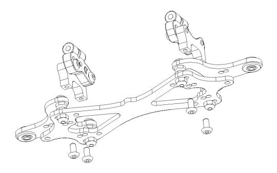
Assembly the 2 groups to the front bear with 4 x HW008 M3x8mm button screw. Use the innermost set of holes.
