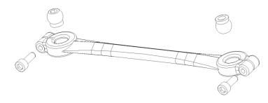
Use 2 x HW0014 M2x 6 screws and 2 x FX002 spheres each
