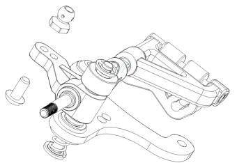
Assembly the FU-FX48 ball stud using the HW-003 M3x8 button screw as shown.
