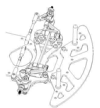
Fix the front end using 4 x HW002 M3 self-locking nut.
