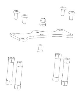
Fix the 4 by 26mm post using 4 x HW003 M3x8 button screw.
