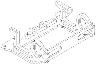
Fix the G56-021 brace to the group using 4 x HW008 M3x6 button screw.
