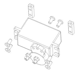
Use the 2 x HW003 M3x8mm button to secure the FX-FU48 to the servo saver.
