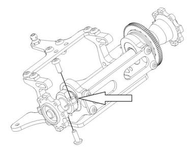
Slide the left hub HDD4 on the rear axle, leave 0.1-0.2mm of axial play. Clamp it on the axle using 2 x HW004 3x10 button screws
