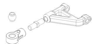
G56-031 arm – G56-033 eyelet-G56-032 turnbuckle G56-037 sphere
