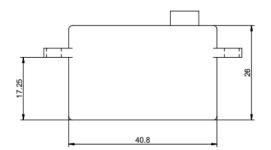
Servo and servo saver are not included, model need a low profile servo.
