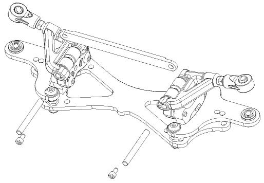
Slide the G56-012 Narrow front beam into the upper arm mounts, then insert the G56-034 hinge pins and secure them with the HW031 M2x4 screw
