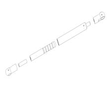
Assembly the 2 side dampers as shown
