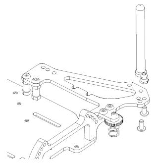
Assembly the FX-FU48 using 1 x HW008 3x6 button screw, the body post using 1 x HW007 3x8 button screw.
