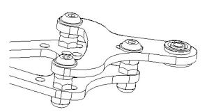
Front end tuning! You can alter the front end rigidity by coupling the front end arms with the front beam.
