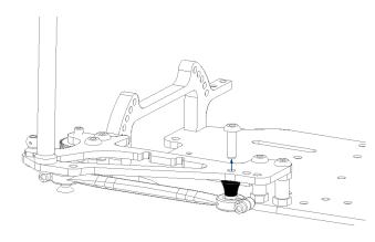
Insert the HW0029 M3x12 in the proper "A" hole, then slide the G56042 spacer Install the link assembled previously
