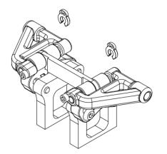
There are4 caster clips, 2 by 1 mm and 2 by 2mm. Those are be used to adjust the static caster.
