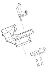
Now you can couple the motor pod to the chassis group. Use the M33-5 shock holder, using 4 by HW008 3x6 button screw.
