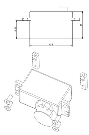
Servo and servo saver are not included, Mistral 3.3 need a low profile or super low profile servo.
