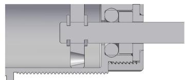
Take care when using conical pistons. As show, the shock will be harder in compression and softer in extension
