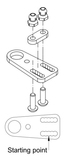
Assembly the steering linkage as shown. Take some care when insert the bearings in the carbon fibre.
