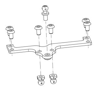
Fix the M33-6 wing stay to the group using 4 x HW008 M3x6 button screw.
