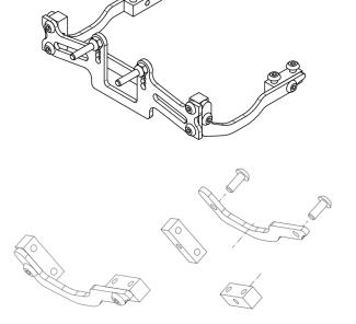
Assembly 2 mirror like shoulders using M20-8 and M20-17 joint. Use 2 x HW003 M3x8 button screw. Do not tight them fully now.
