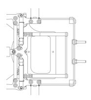
Use 4 x HW003 M3x8 button screw and assembly the M20-6 wing holder to the shoulders Do not tight them fully now.
