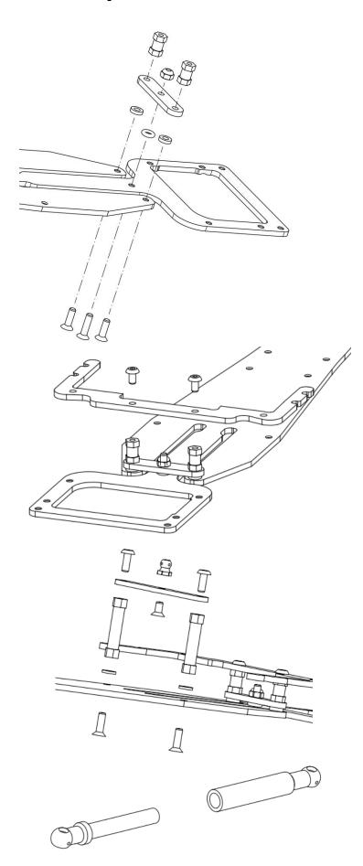
Start with the HW026 M3x12 countersunk and insert it in the central hole of the "T-bar", slide the o-ring over it.
