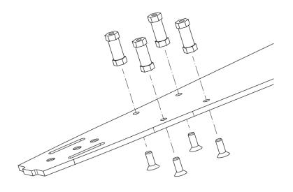
Fix the 4 x FX1049 15mm post to the chassis using 4 x HW007 M3x8 countersunk.
