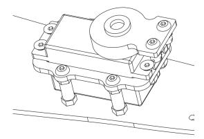
Install the servo group using 4 x HW003 M3x8 Button
