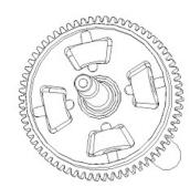
Install the 4 pinions. Start with a 50K – 100K grease, better results are achieved by using a grease with a good thermal stability
